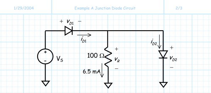
1) If 6.5 mA flows through a 0.1 K resistor, the voltage across that resistor is:
